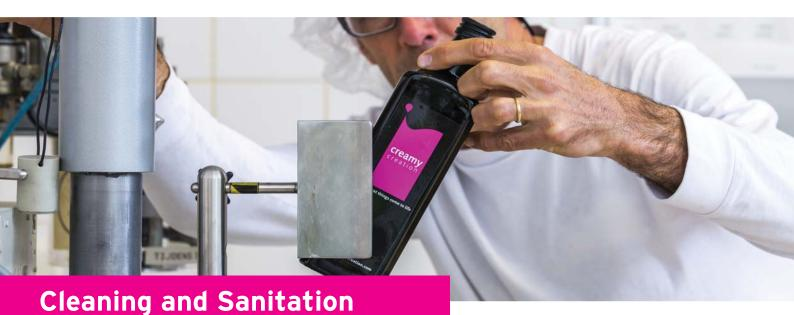
One of the principal concerns of manufacturers and bottlers of cream liqueurs is plant cleanliness and hygiene. While distilled spirits and cream liqueurs do have a sterilizing effect, it is important to understand that after emptying a tank, line or filler, some product will remain. From these remains the alcohol can evaporate rapidly and the residue becomes sensitive to micro-organisms. Improper equipment cleaning may compromise the next batch produced.
